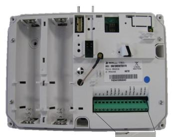
Prog. Out. COM When triggering an external hardwired Prog. Output2 device you must be hooked up here. Prog. Output1 Ref GND Prog. Input3 Prog. Input2
